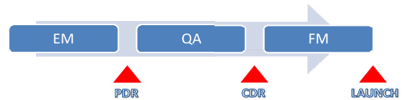
Fig. 20. Process plan for the construction of the CanSat
