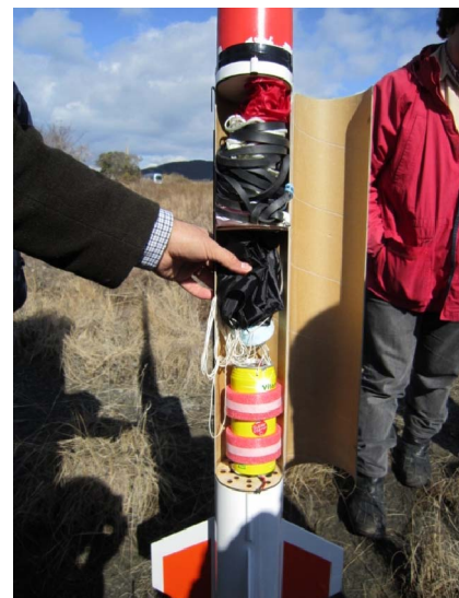
Fig. 2 CanSat packaging inside the rocket just before the launch
