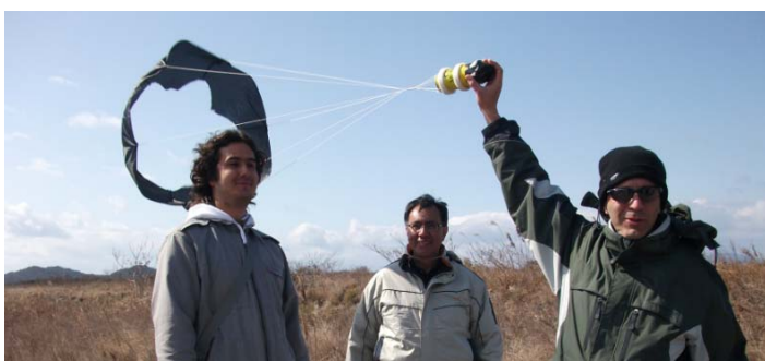
Figure 3. Ground testing the CANSAT assembly parachute in high winds
